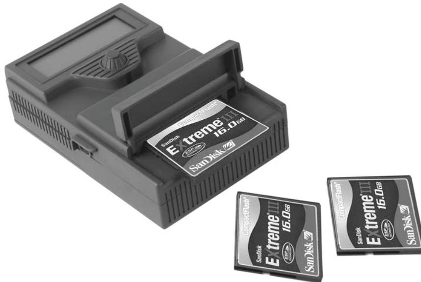
**1. CF Card Protection Cover** – Slide down then lift up carefully to open this cover and get access to the CF card slot and the card eject button.
